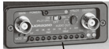
Typical transmitter gain control with LEDs for adjustment.
