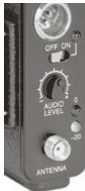
Typical transmitter gain control with LEDs for adjustment.
