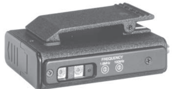
Two 16-position rotary switches adjust the operating frequency of the transmitter over a 25.6 MHz bandwidth in 100 kHz steps.
