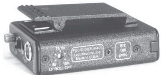
The low frequency roll-off is adjustable from 35 Hz to 150 Hz to control the presence of extremely low frequency audio in the program material.
